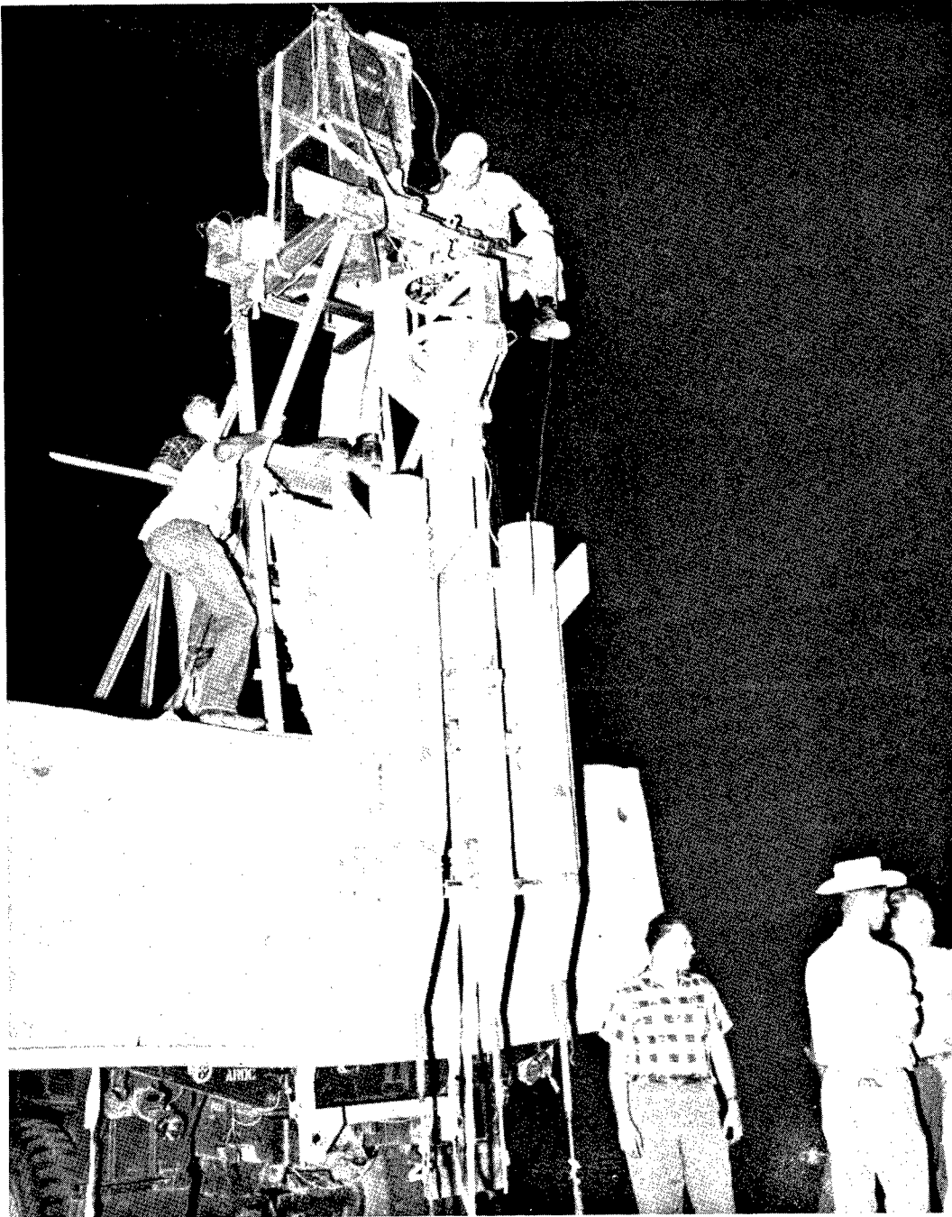
Cree Missile Cluster, Especially Developed for Parachute Experimentation, Being Prepared for Balloon Drop Test
